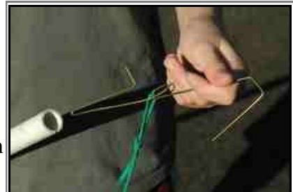
Figure 1: A wire coat hanger bent into this hook and loop shape makes raising that EmComm or Field Day antenna much easier.
